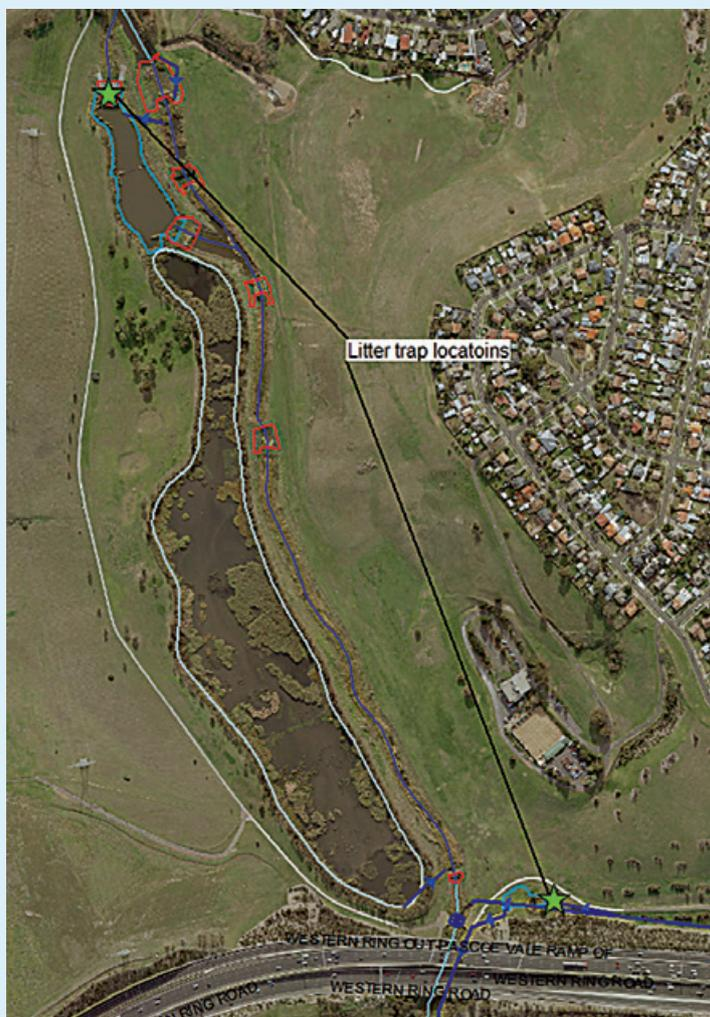
Both these litter traps provide a significant amount of litter treatment. However during large storm events they are unable to treat all the water that is flowing through the system and this is causing the build-up of litter and debris at the bridge.
