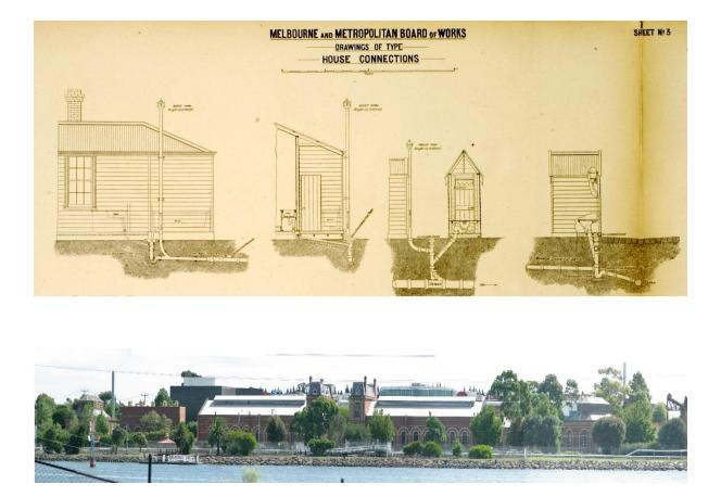
Figure 31. Detail for house connections into sewerage only system. Spotswood pumping station beside the Yarra. Sources: PROV, VPRS 8609/P20, Unit 332 – Author photo (2015).
