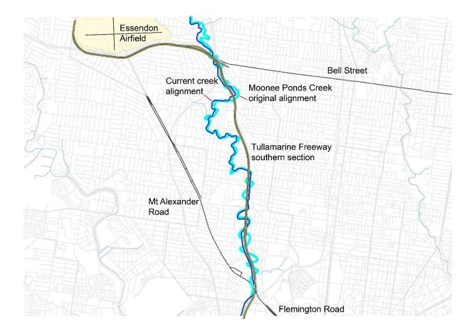
Figure 93. Original creek alignment in aqua with current alignment in blue, overlaid with the freeway route.
