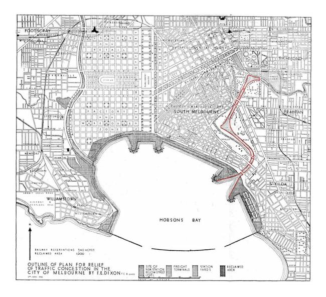
Figure 46. Dixon's plan for realigning the Yarra - the new river course marked in red. Source: Dixon (1944).
