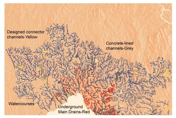
*Figure 56. Melbourne's underground main drains, concrete-lined watercourses and constructed connector channels that transfer flood flows between creeks.*
