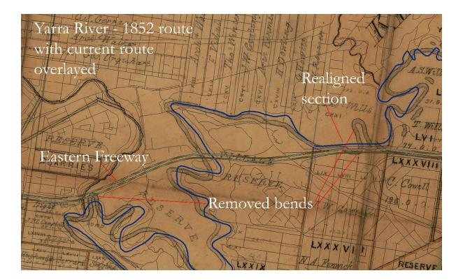
Figure 102. Modifications to the Yarra for the freeway.
