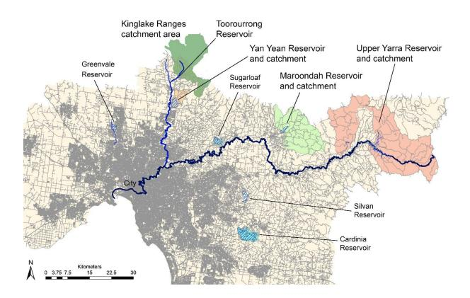
Figure 18. Melbourne's closed water catchments and main reservoirs. Suburban reservoirs have no or limited catchments and filled by conduit from outer reservoirs.
