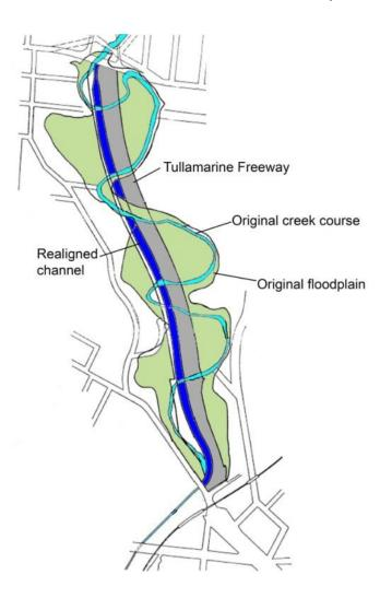
Figure 95. Plan showing the area of floodplain lost due to construction of the freeway. Source: MMBW (1981).
