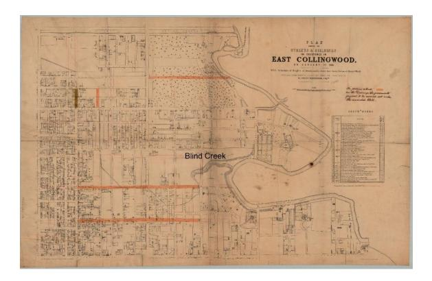
Figure 100. Blind Creek in 1858, showing the upper reaches either changed into lined channels or undergrounded into barrel drains. Source: SLV http://handle.slv.vic.gov.au/10381/117381
