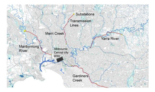
Figure 67. High voltage power transmission lines along watercourses.
