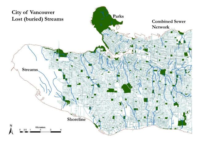
Figure 33. City of Vancouver buried streams in relation to combined sewer mains.
