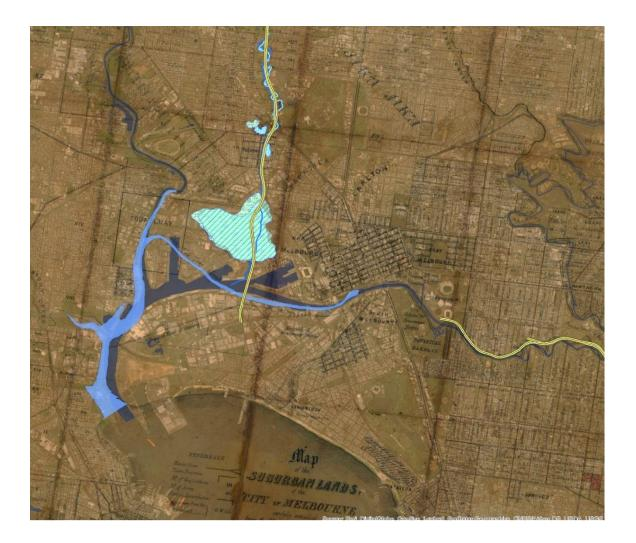
Figure 97. The location of CityLink, Western Link, joining the end of the Tullamarine with the West Gate. The link covers sections of the Moonee Ponds, crosses reclaimed land of the West Melbourne Lagoon, and the Yarra to join with the West Gate (not shown) The freeway to the right is the South-Eastern (Monash) ending where it enters a tunnel. The map also shows the original course of the Moonee Ponds and the Yarra.
