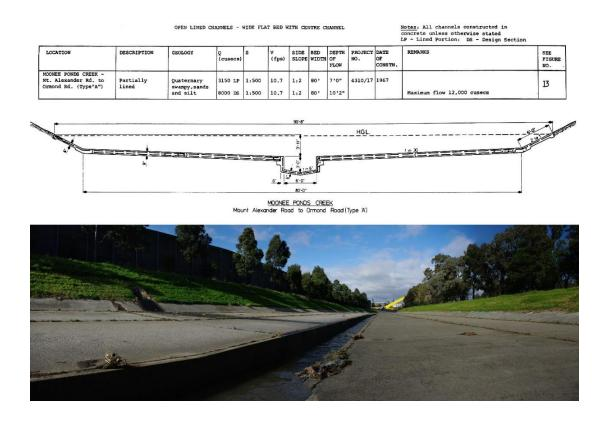
*Figure 53. Section Moonee Ponds Creek realigned for the freeway. Source: MMBW (1980) and Author photo (2016)*
