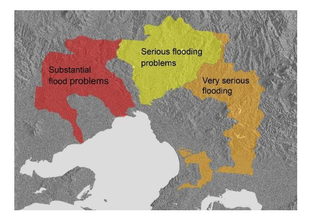
Figure 86. Flooding classifications of the MMBW 1971 Planning Policies, based upon topography, level of control works and scale of flooding. Source: MMBW (1971).
