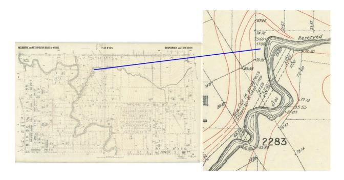
*Figure 110. MMBW 1907 plan showing proposed straightening of a section of Melville Creek in Brunswick. Source: SLV http://handle.slv.vic.gov.au/10381/143010*
