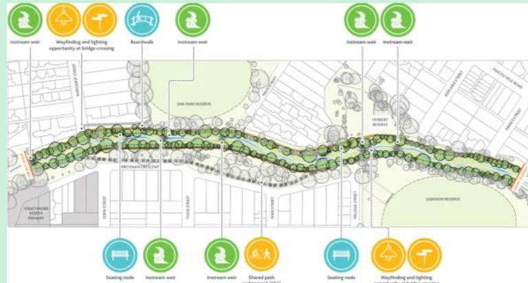
**Design Concept A** includes an upgrade of the creek channel from where the concrete starts to beyond Marks Street. The design involves limited re-engineering of the channel, replicating the current creek layout. However this option creates 650m length of naturalised waterway as opposed to 500m for options B and C.
