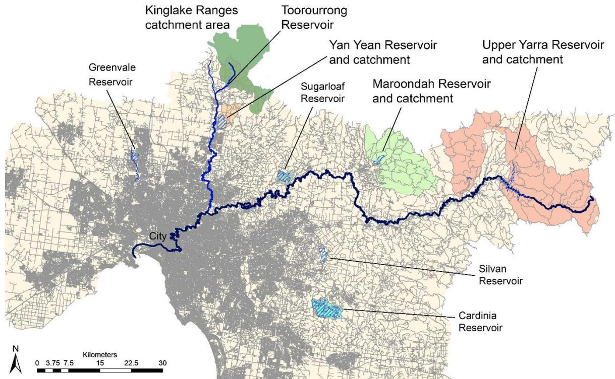
Figure 18. Melbourne's closed water catchments and main reservoirs. Suburban reservoirs have no or limited catchments and filled by conduit from outer reservoirs.
