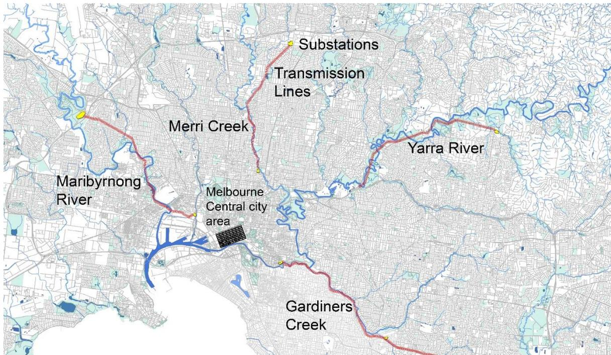
Figure 67. High voltage power transmission lines along watercourses.
