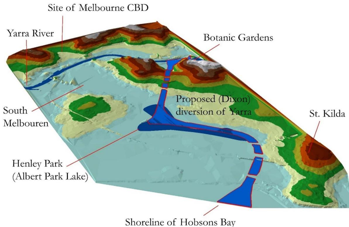
Figure 47. Model of Dixon's proposed scheme cutting through the ridge and Botanical Gardens.
