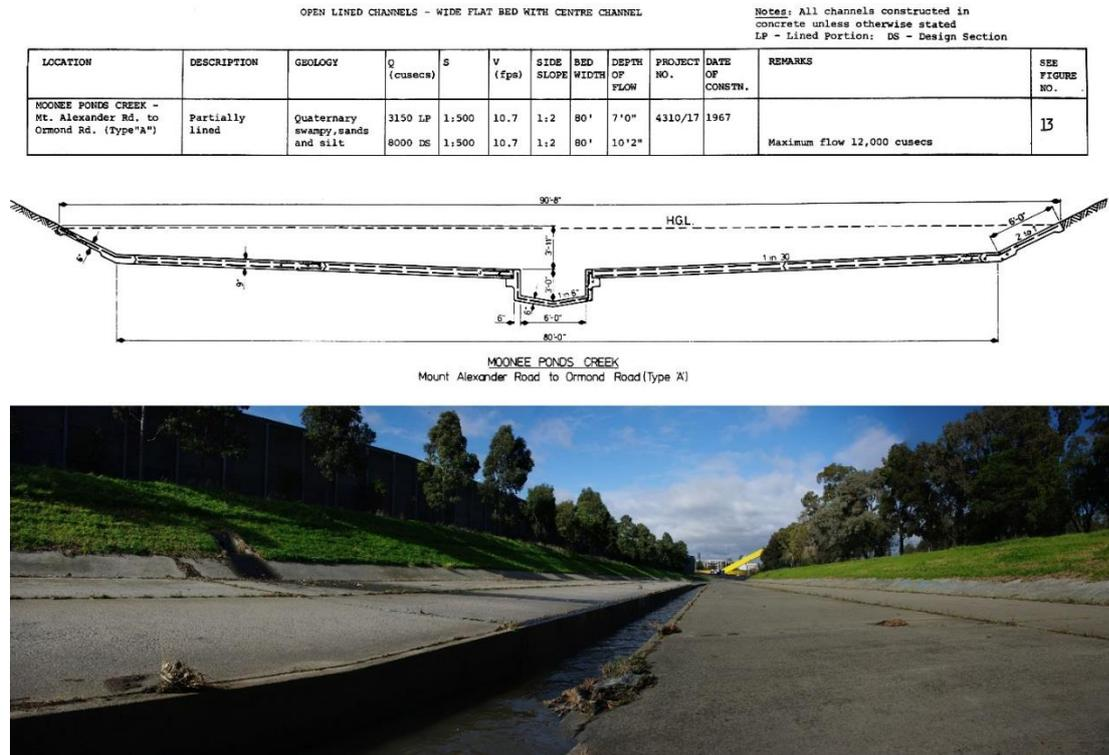
Figure 53. Section Moonee Ponds Creek realigned for the freeway. Source: MMBW (1980) and Author photo (2016)
